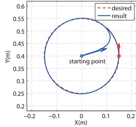
Fig. 5. Desired and actual trajectories of the circular path tracking task, where the robot and human hand start from the center of the circle.
