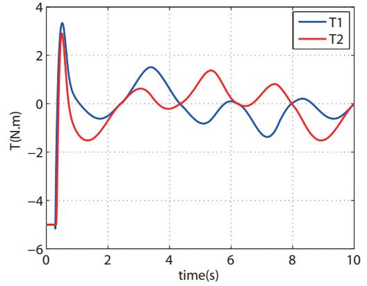
Fig. 7. Torque inputs of the robot based on PD-computed torque controller, and the maximum motor torque is 5 N.m in the simulation.
