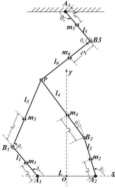
Fig. 4. Diagram of the human-robot system, and definition of the dynamics parameters.
