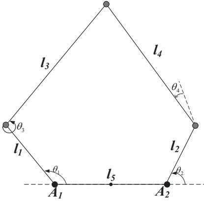
Fig. 2. Two-DOF parallel mechanism.
