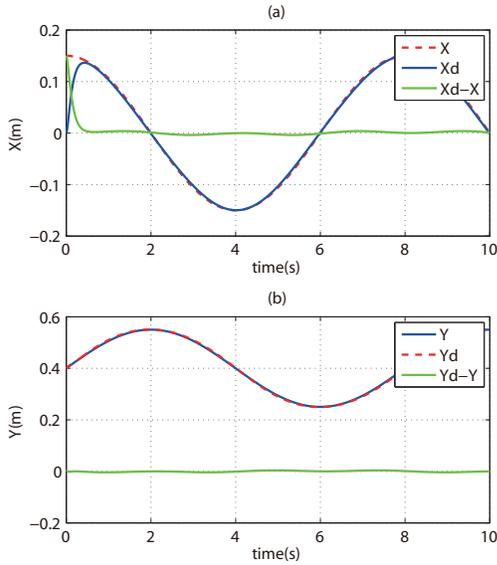
Fig. 6. Desired and actual trajectories, and tracking errors in X and Y directions.
