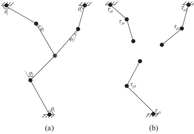
Fig. 3. Two-DOF redundant parallel mechanism and its equivalent open-chain system.
