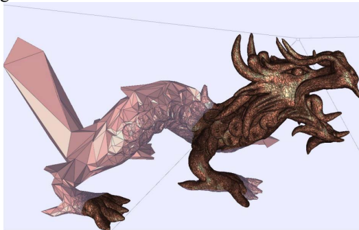
Figure 4. Illustration of Random accessible mesh from [36]. Note that different part of the dragon can be displayed in different resolution.
