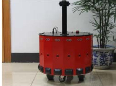
Fig. 5. The experiment robot AIM. Diameter D_r = 48cm .
