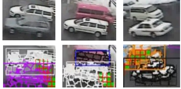
Figure 3: Sample results of semantic superpixel propagation when detectors lose effectiveness (1st row: source images; 2nd row: the propagation results).
