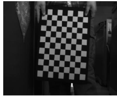
Fig. 4 The planar calibration target
