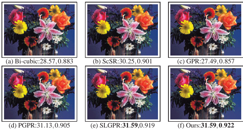
Figure 3: Comparison of SR results ( \times 2 ) on flowers image. (a) Bi-cubic interpolation. (b) ScSR method [15]. (c) GPR method [5]. (d) PGPR method [8]. (e) SLGPR method [7]. (f) The proposed method. The two numbers below each figure are PSNR and SSIM respectively.
