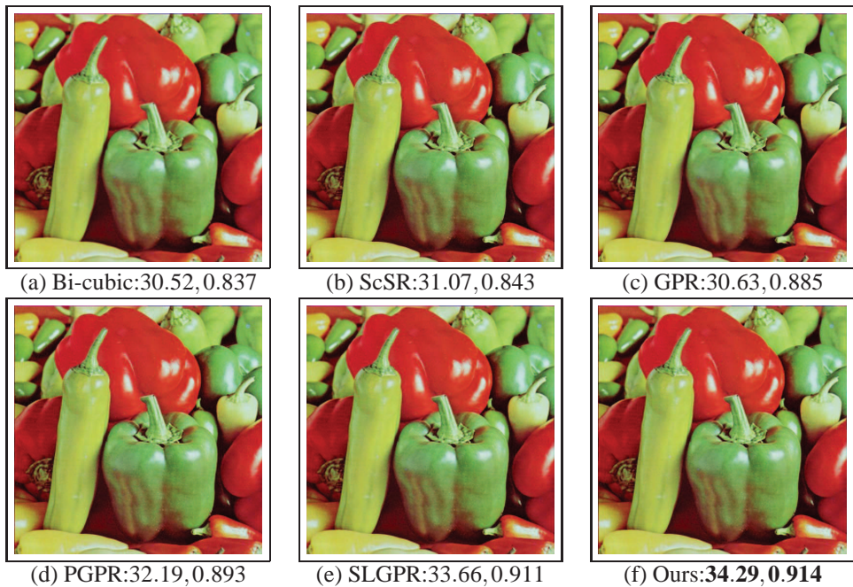
Figure 2: Comparison of SR results ( \times 2 ) on Pepper image. (a) Bi-cubic interpolation. (b) ScSR method [15]. (c) GPR method [5]. (d) PGPR method [8]. (e) SLGPR method [7]. (f) The proposed method. The two numbers below each figure are PSNR and SSIM respectively.
