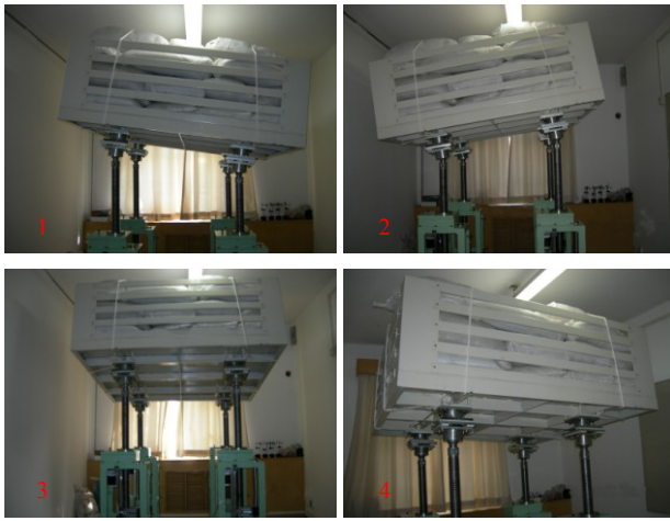
Fig. 8 Tectonic deformations (1 – left incline, 2 – right incline, 3 – forward incline, 4 – diagonal incline)
