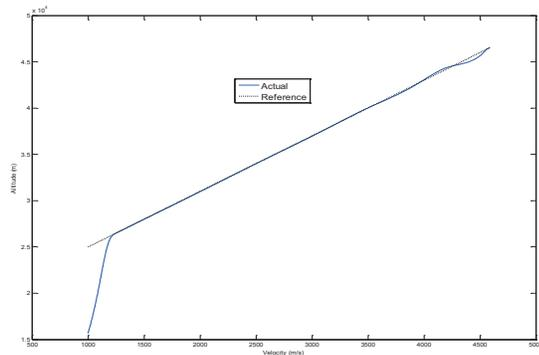
Fig. 7 Entry trajectory with the final velocity changed to 1000 m/s
