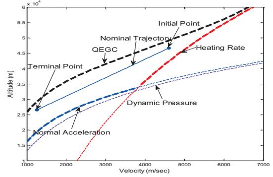
Fig. 2 Entry corridor and the nominal trajectory
