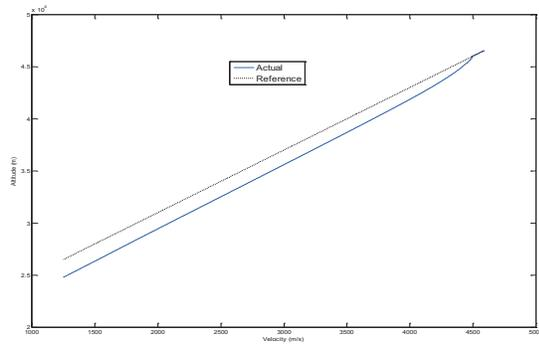
Fig. 6 Entry trajectory with the altitude integrator cancelled
