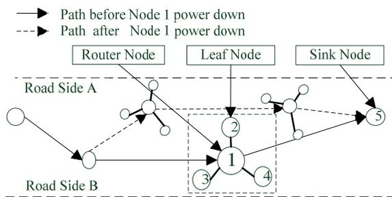
Figure.5. WSN for BRT Signal Priority
