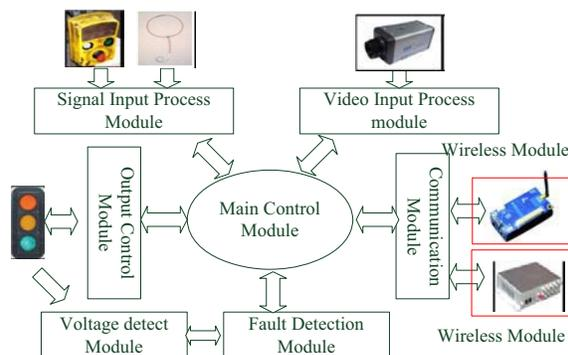
Figure.9 Signal Priority Supported Traffic Signal Controller
