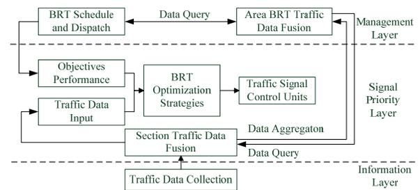
Figure.3. Transit Signal Priority Systems Architecture
