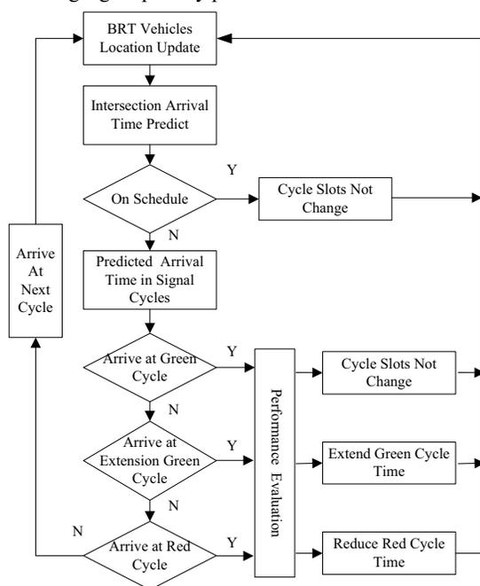
Figure.4. BRT Signal Priority Process
