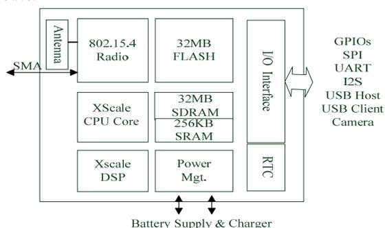
Figure.7. Video Sensor Node Hardware
