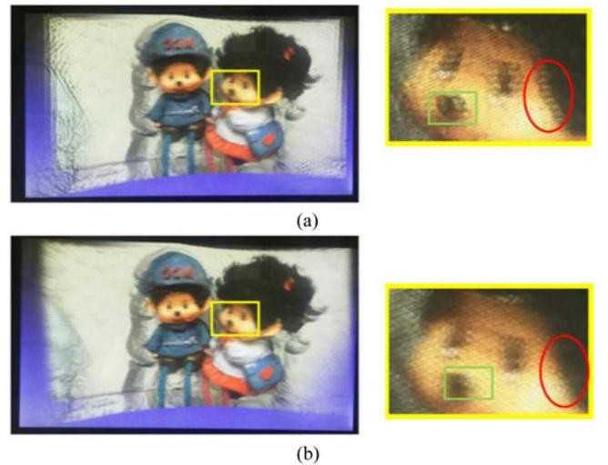
Fig. 7. The synthetic image of a scene “Mccs” observed at one optimal viewing position. (a) Result of 9-view display. (b) Result of 27-view display.
