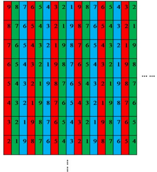
Fig. 1. The result of traditional mapping process for 9-view display.
