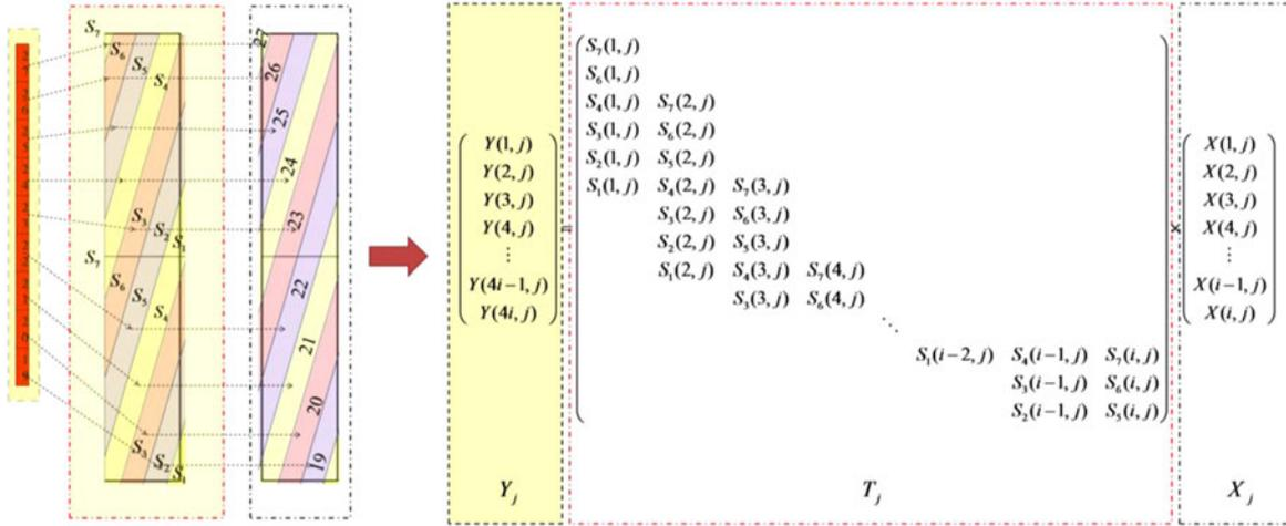
Fig. 6. The formula for multiplexing process. After the multiplexing, viewers will observe “mix up” subpixels from the lenticular sheet as if they see the corresponding view images’ subpixels.
