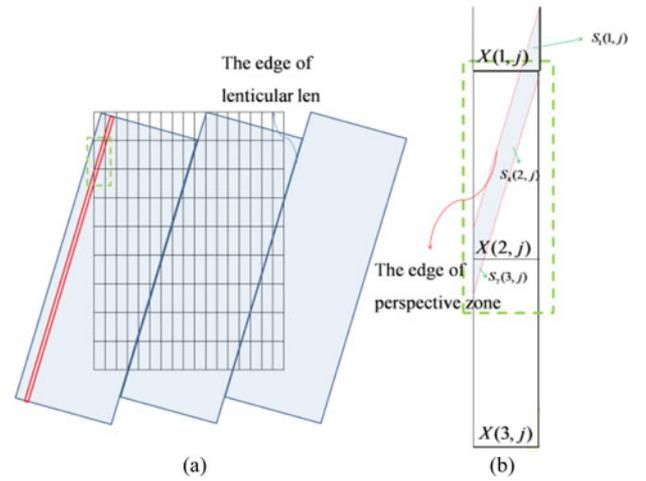
Fig. 2. (a) One of the perspective zone on the lenticular sheet illuminated with red color is prepared for the observer at the 21st optimal viewing position. Blue and red lines represent the edges of lenticular lens and perspective zones respectively. (b) The shape subpixel in the perspective zone observed through the lenticular sheet is a parallelogram but not a rectangular.
