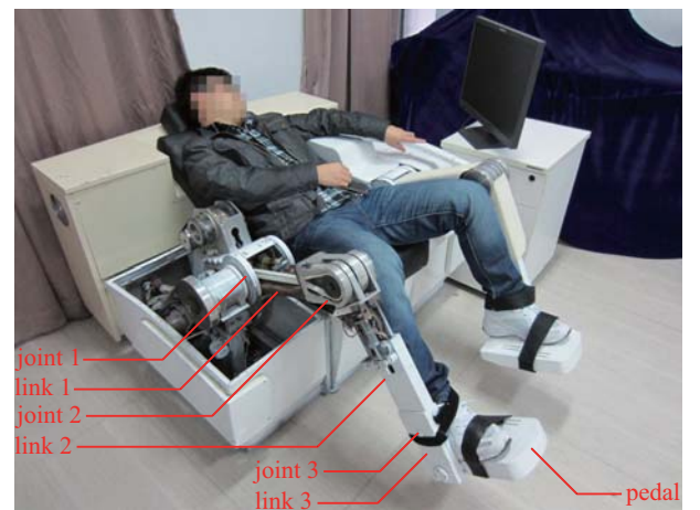
Fig. 1. Mechanical structure of iLeg for lower limb rehabilitation
