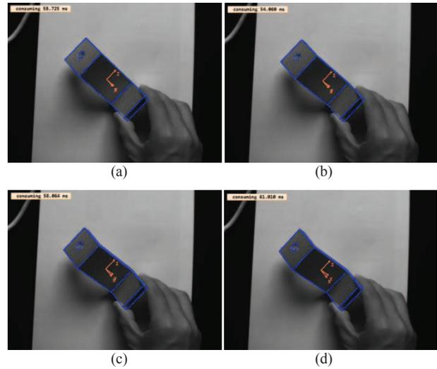
Fig. 6. The bracket can be tracked successfully with the proposed approach. (a)-(d) show tracking results for the metal bracket. The pose of the bracket is visualized by the blue edges, and the consuming time of each frame are listed.
