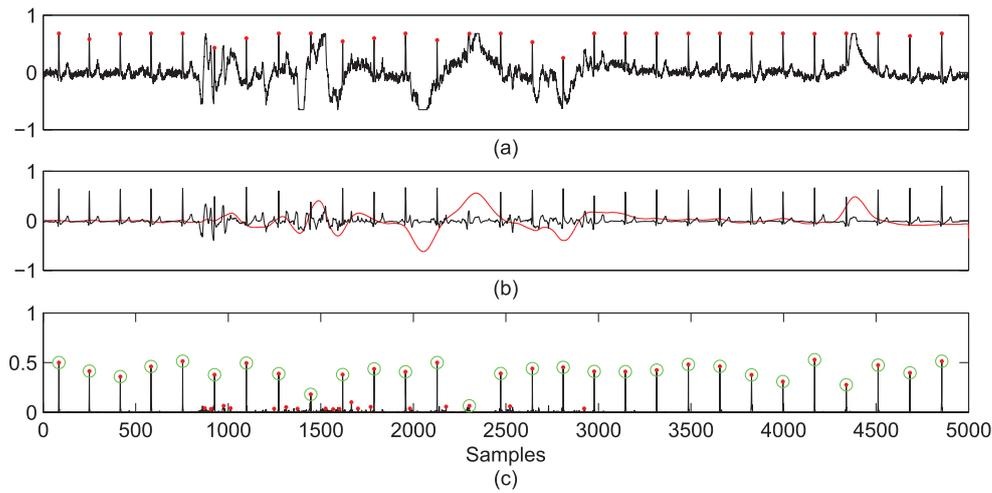
**Figure 4.** ECG enhancement and QRS complex detection. (a) ECG recording s00377 from PhysioNet MIMIC II waveform database matched subset; (b) denoised ECG signal and removed baseline; (c) reconstructed QRS peak information signal, local maxima points (denoted by red dots) and detected QRS complex locations (denoted by green circles).
