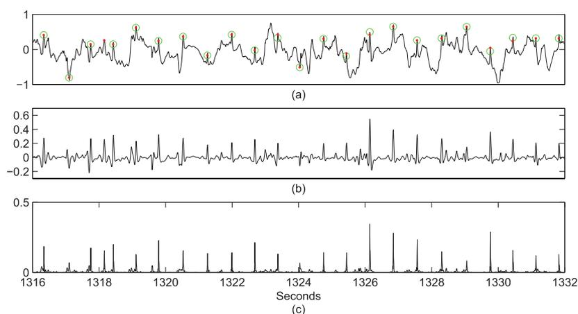
**Figure 7.** Denoised and QRS detected version of record 105 in MIT-BIH database. (a) Input ECG recording from 1316 to 1332s; (b) denoised and baseline-corrected ECG signals derived using our proposed algorithm 1; (c) reconstructed QRS peak information signal. Note that in (a), the entire signal was normalized between  $-1$  and  $1$ , and the detected and reference annotations are marked using red dots and green circles, respectively.
