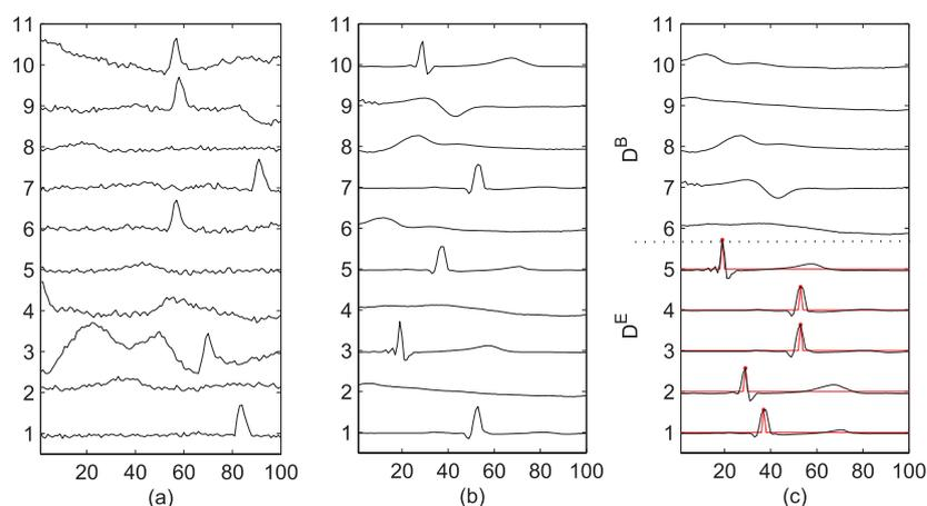
**Figure 2.** Examples of training set and learned dictionary: (a) examples of raw signal segments used in the training set; (b) some atoms selected from the dictionary that were learned from the training set; (c) selected atoms from the separate sub-dictionaries (denoted by  $D^B$  and  $D^E$ ). Noted that the atoms labeled in (b) correspond to the atoms labeled in (c).
