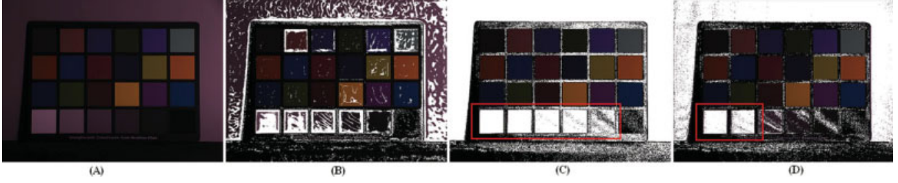
FIG. 3. An example of achromatic surface identification. The white color means these pixels are achromatic. (A) is original image. (B) is the identification result after first iteration of CCAS (optimized), pixels identified as achromatic are indicated in white. (C) is the final identification result using optimized initial condition. (D) is the final identification result iterations using original CCAS, pixels identified as achromatic are indicated in white.
