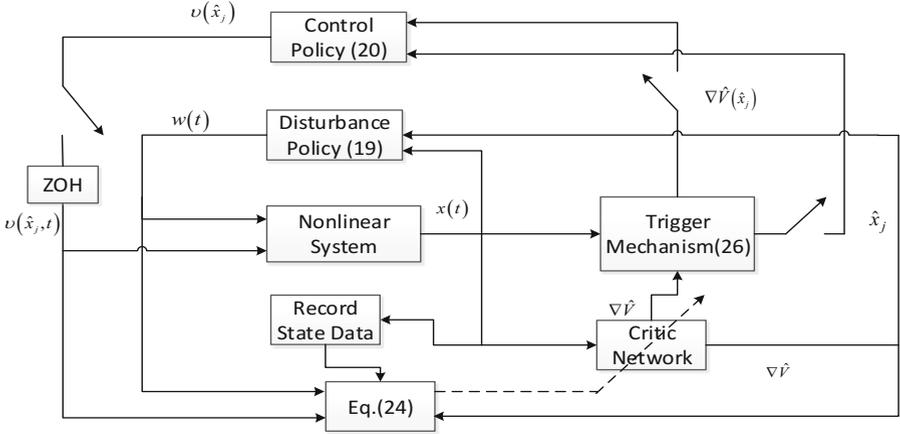
Fig. 1. Structure diagram of the ETCL algorithm for two-player ZS game
