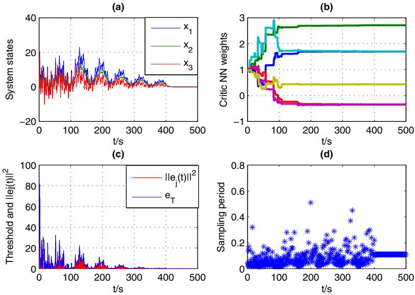
Fig. 2. (a) Evolution of system states. (b) Convergence of the critic parameters. (c) Triggering threshold  $e_T$  and  $\|e_j(t)\|^2$ . (d) Sampling period.
