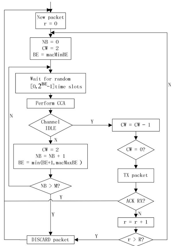
Fig. 1. Flowchart of the channel access procedure
