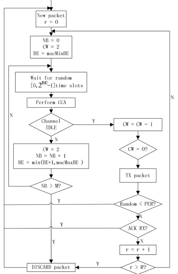
Fig. 3. Flowchart of the revised channel access procedure
