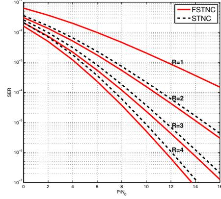
Fig. 3. SER performance comparisons between the proposed FSTNC scheme and the conventional STNC scheme.
