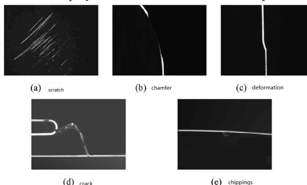
Fig. 2. typical defects on cover lens of touch screen
