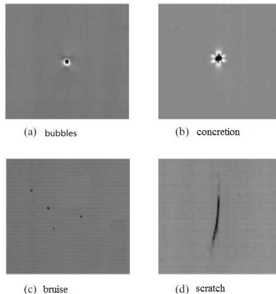
Fig. 3. typical defects on float glass surface
