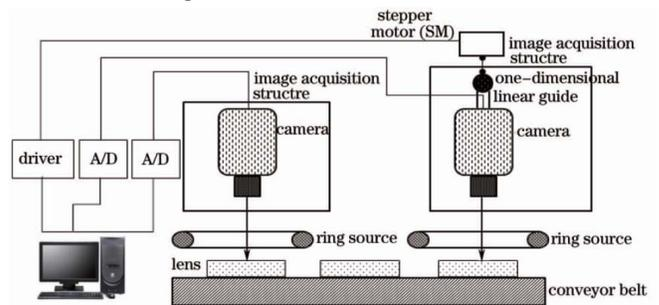
Fig. 7. Schematic diagram of the system
