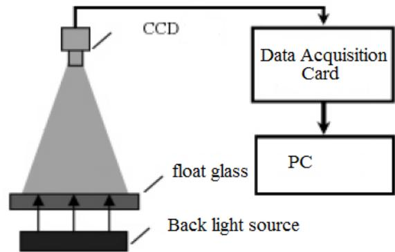
Fig. 6. typical inspection system
