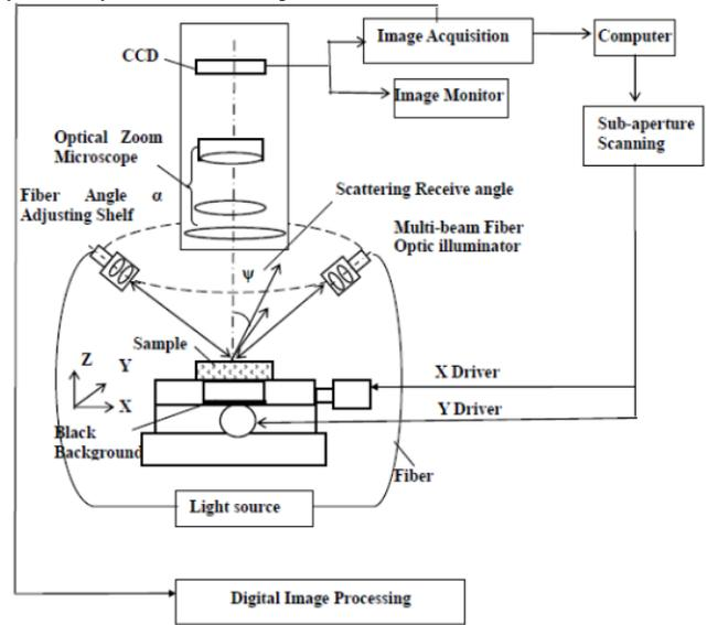
Fig. 5. Microscopic Scattering Imaging System
