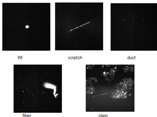
Fig. 1. typical defects on the optical element surface
