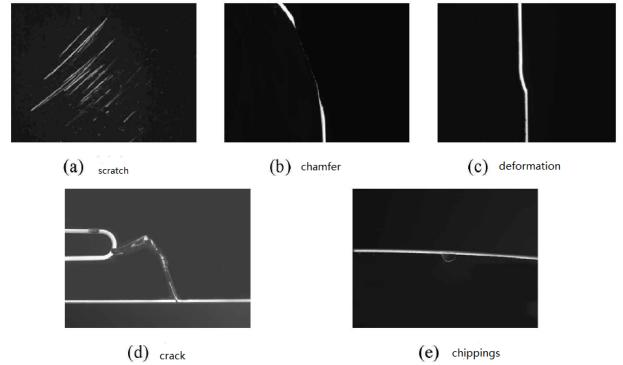
Fig. 2. typical defects on cover lens of touch screen
