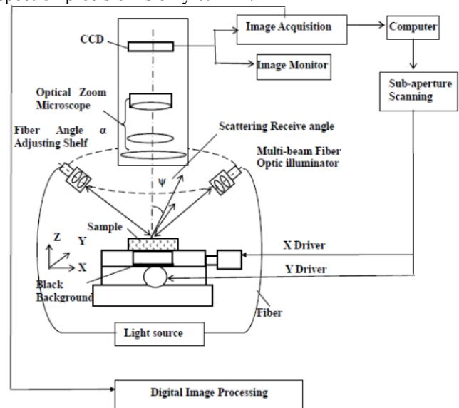
Fig. 5. Microscopic Scattering Imaging System
