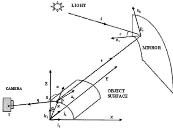
Fig. 10. illumination system structure
