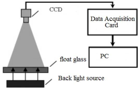
Fig. 6. typical inspection system
