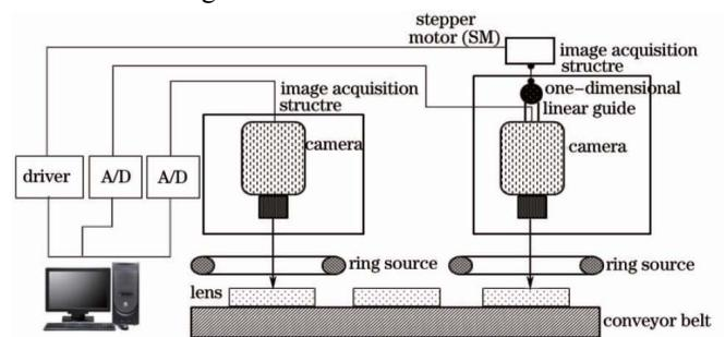
Fig. 7. Schematic diagram of the system
