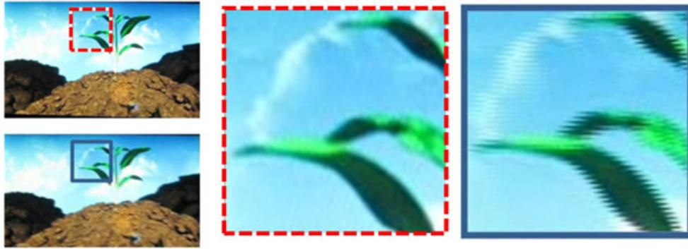
**FIGURE 9** — Lower left panel and enlarged right panel: without optimization, corresponding to point “d” in Fig. 8(a); Upper left panel and enlarged center panel: proposed optimized crosstalk reduction method, corresponding to point “c” in Fig. 8(c).
