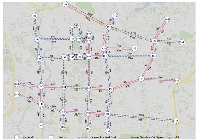
Fig. 3. Optimal sensor locations (sensor number=56, sparse degree=28).
