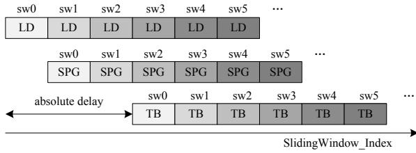
Fig. 3 Viterbi decoder pipeline sequence
