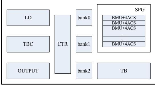
Fig. 2 reconfigurable viterbi decoder function frame
