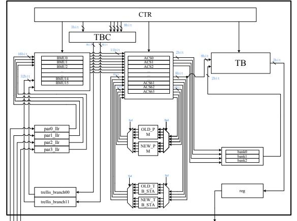
Fig. 5 the circuit architecture of Viterbi decoder
