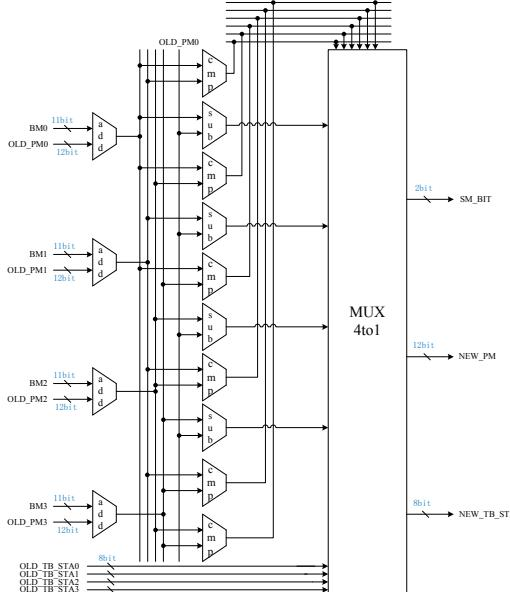
Fig. 7 ACS unit structure under Radix-4 algorithm
