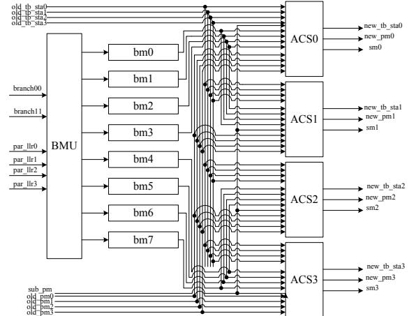
Fig. 8 the circuit structure of SPG
