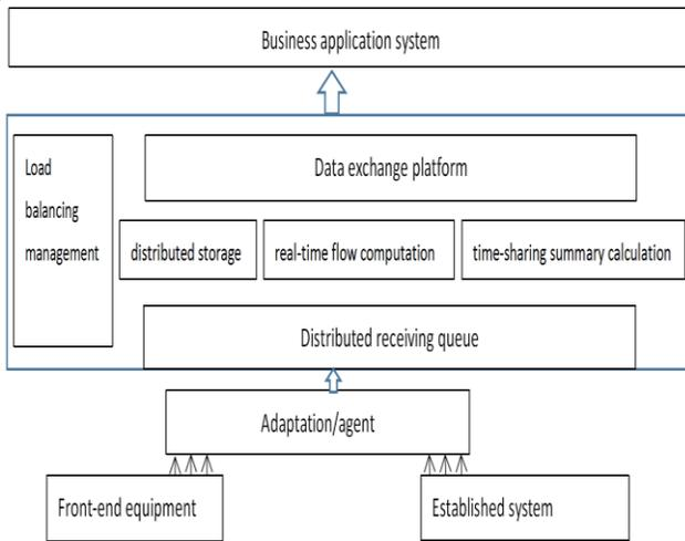
Fig. 4. Traffic data processing architecture
