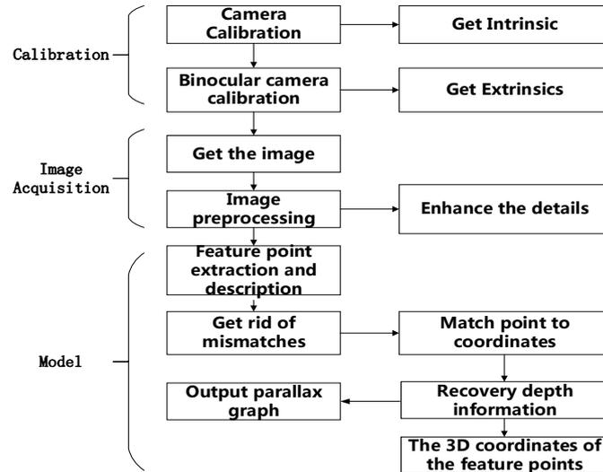
Fig. 3. A flow chart of 3D reconstruction based on machine vision technology
