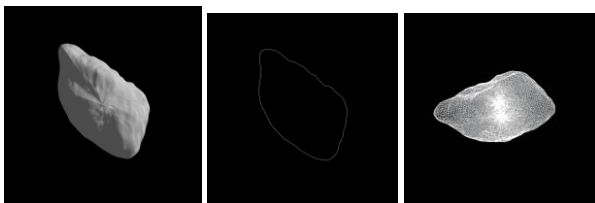
(a) Simulated image (b) Contour of the target (c) Matched template Fig. 8 The process of LOS determination:
