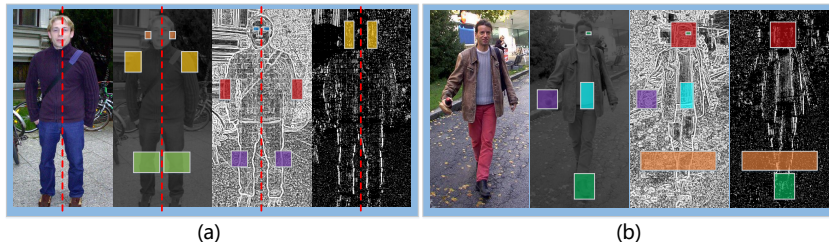
Figure 1: (a) Symmetric features. For clarity, we just show three channels (L channel, gradient magnitude, and one gradient orientation) here. Rectangles with the same color in the same channel represent one symmetric feature. (b) Cross-channel features. Rectangles with the same color in different channels represent one cross-channel feature.
