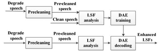
Figure 3: Block diagram of the proposed LSFs enhancement
