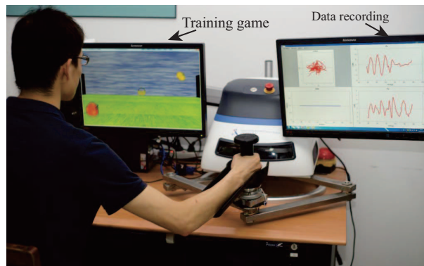
Figure 1 (Color online) Training scenario using CASIA-ARM, where the patient is directed to catch the moving objects in the virtual environment with the robot's assistance.
