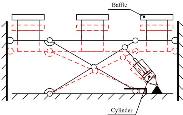
Fig 8. Scissor lift mechanism structure
