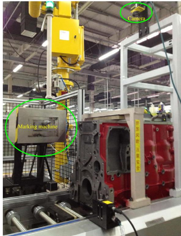
Fig 5. Cylinder block type identify and QR code marking
