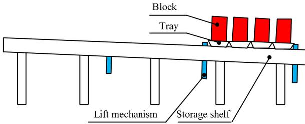
Fig 7. Cylinder block segmented storage scheme
