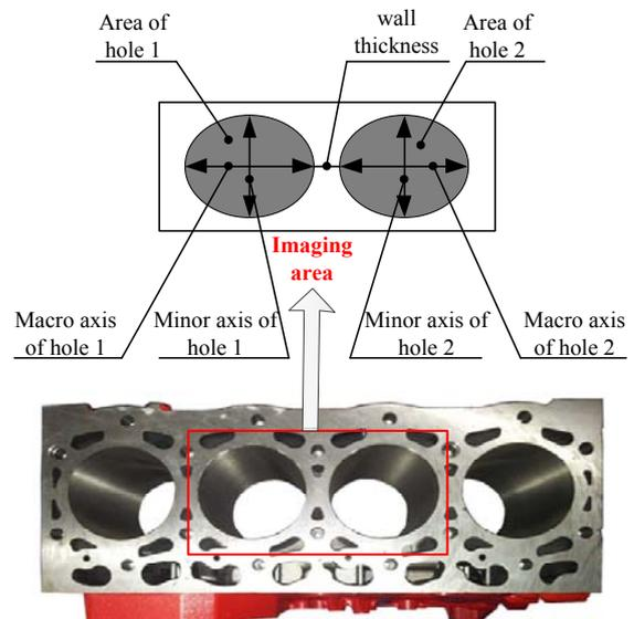
Fig 3. Cylinder bore image recognition solution
