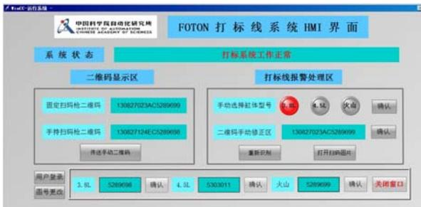
Fig. 11 Type identify and mark system interface
