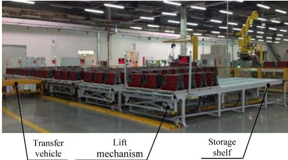
Fig. 12 Automatic logistics system application
