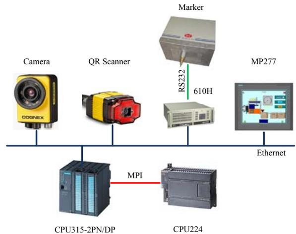
Fig 2. Hardware connection of the control module
