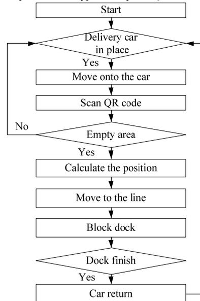
Fig 6. Cylinder block automatic storage flowchart
