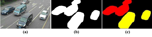
Fig. 3. The motivation of RSCH method. (a) Current frame, (b) foreground, (c) the yellow region represents total occlusion or no occlusion, and the red region means partial occlusion. In (c), when occur total occlusion or no occlusion, each connected region is a convex set or approximate to a convex set when total occlusion or no occlusion occur. However, it will be very different when some vehicles with partial occlusion.
