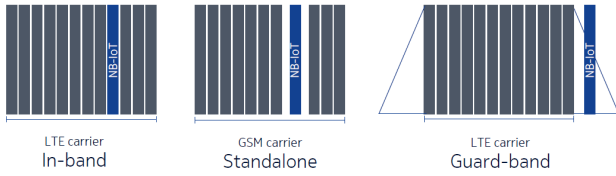
Fig. 1. The deployment options of NB-IoT.
