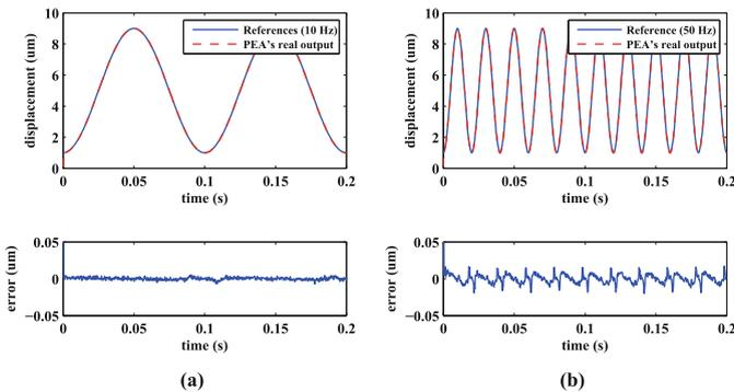
**Fig. 2.** Tracking performance of the PEA under different references: (a)  $10\ \text{Hz}$ ; (b)  $50\ \text{Hz}$ .
