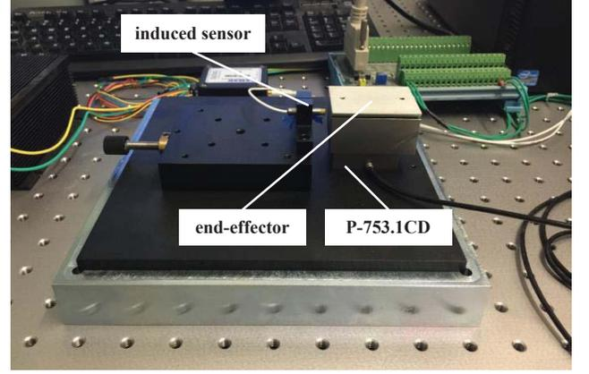
Fig. 3. The prototype of the piezoelectric-actuated stick-slip device developed in [31].
