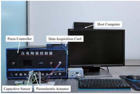
Fig. 4. The self-developed controller for PEAs.
