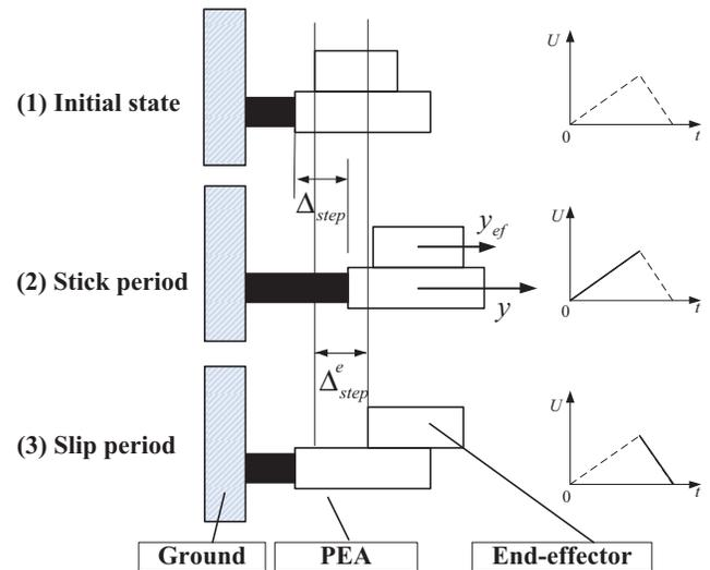
Fig. 1. Working principle of the piezoelectric-actuated stick-slip device [4].
