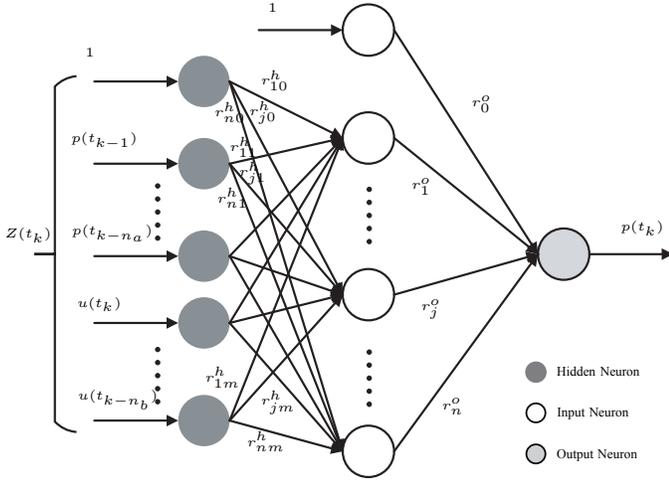
Fig. 2. Structure of the three-layer feedforward neural network for modeling the piezoelectric-actuated stick-slip device [31].
