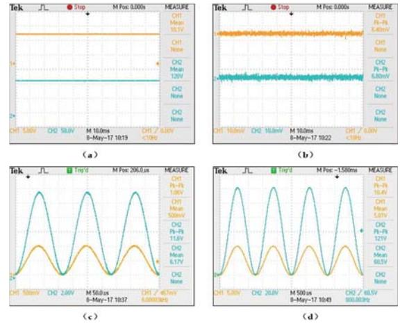
Fig. 5. Controller performance test: (a) DC voltage; (b) static ripple; (c) sinusoidal output with low peak-to-peak voltage; (d) sinusoidal output with high peak-to-peak voltage. (Tektronix TDS 2024C digital oscilloscope)
