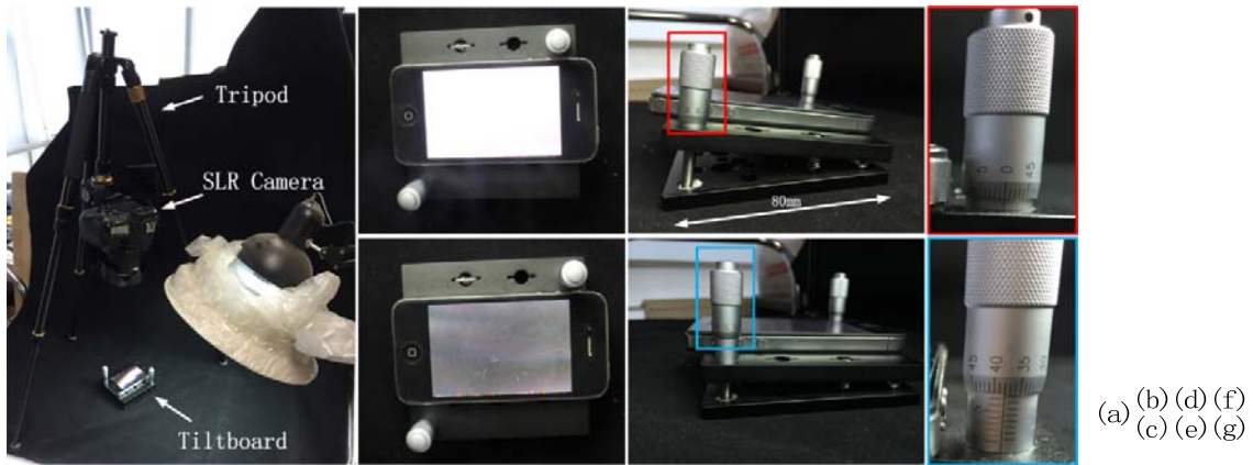
Figure 6. (a) The Experimental platform for FOV evaluation: the digital SLR camera is 300mm distant from the mobile. We first set the differential head as 0 mm ((d)), where a “brightest” picture can be seen. Then we adjust the differential head until the “darkest” picture appears ((c)) and the degree scale of the differential head is 7.88mm ((e)).
