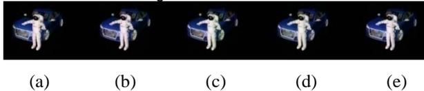
Fig. 10 double-layer diffusing screen different  $N_{view}$  value effect (a)  $N_{view} = 49$  (b)  $N_{view} = 99$  (c)  $N_{view} = 149$  (d)  $N_{view} = 199$  (e) is not segment
