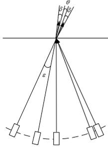
Fig. 3 Diffuser angle and the relative positions among projector units of the projectors
