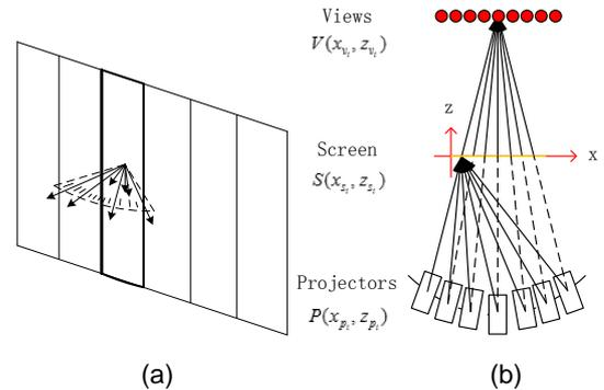
Fig. 5 (a) shows the area of the block and the projector light emission direction. (b) Split splicing simulation of light field reconstruction algorithm.
