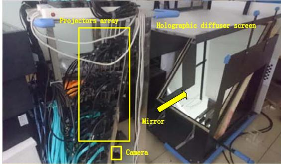
Fig. 2 System structure diagram and the hardware
