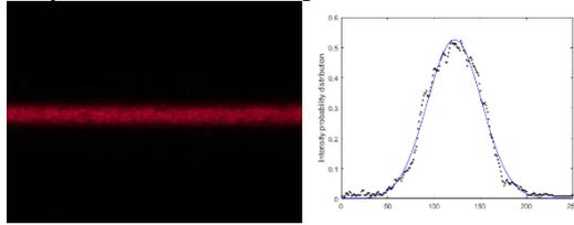
Fig. 8 (a)The laser is shot through the light bar after the scattering screen. (b)Light intensity distribution and Gaussian fitting results.
