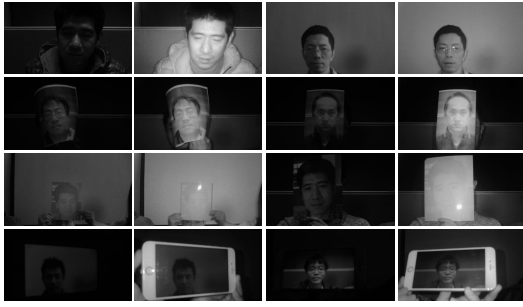
Figure 4. Some samples in our NIRD image datasets. Images from top row to down are genuine faces, A4 paper photos, RC paper photos and tablet screen photos respectively. The first and third columns are NIR images, and the second and fourth columns are NIRL images.
