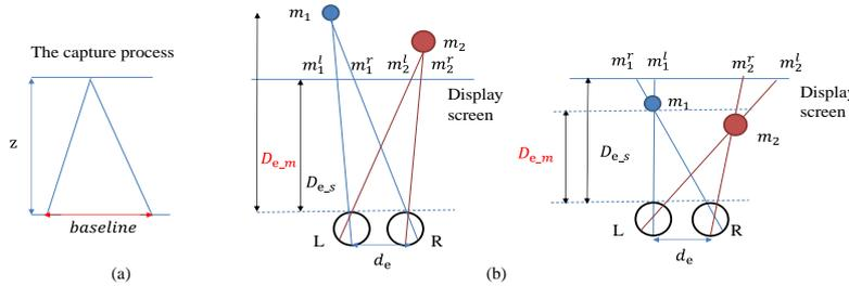
Fig 2. (a). The capture process when acquired the RGBD images; (b). Depth scenes' calculation:  $D_{e,s}$  and  $D_{e,m}$  represent the distances between viewer's eyes to screen and to displayed object  $m_1$ , respectively. And  $S$  is the display scale between the display image size and the original view image size.
