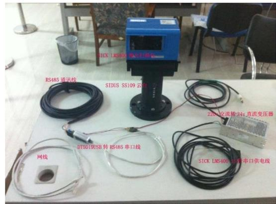
Fig. 7 Hardware components
