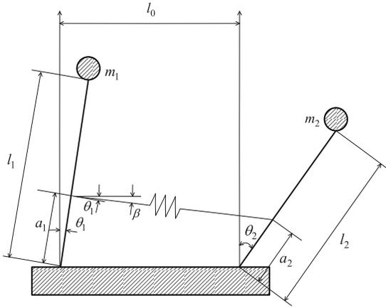
Fig. 4. Parallel inverted pendulum system.
