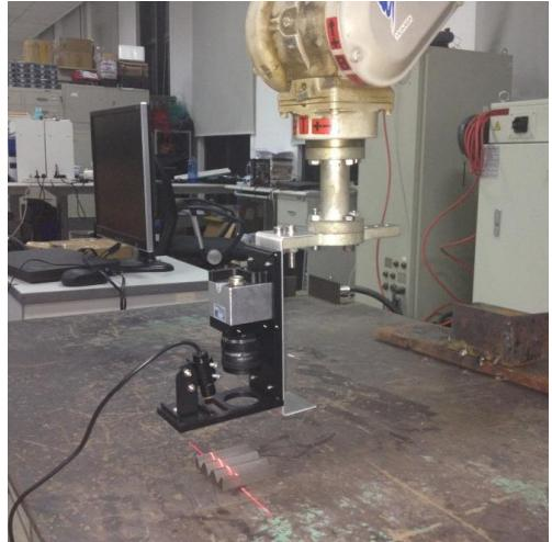
Fig. 9: The experiment scene of the structured light vision measurement on multiple V-shape target
