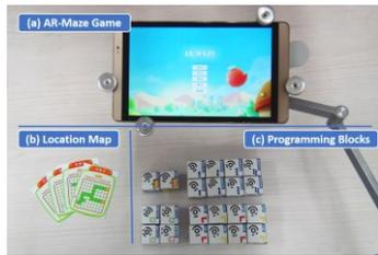
Figure 2: AR-Maze is composed of a) AR-Maze Game, b) Location Map, c) Programming Blocks.
