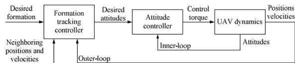
Fig. 1. The two-loop control structure scheme for an UAV.
