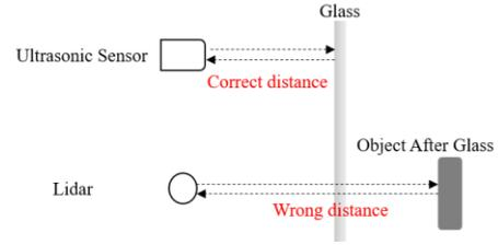
Figure 3. Robot sensors detect glass.
