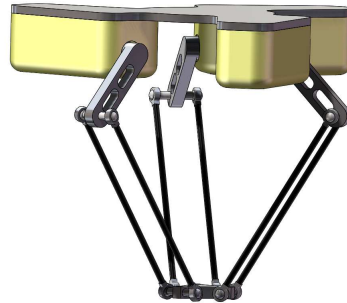
Figure 1. Schematic of a Delta robot.
