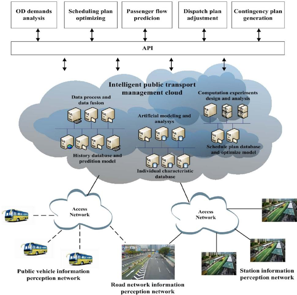
Fig. 2. Parallel transportation management system based on intelligent traffic clouds.
