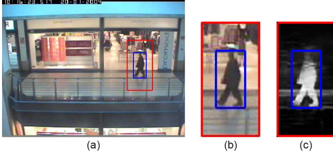
Fig. 1. Example of weight calculation with the guided filter (a) Input frame. (b) Target and its local background rectangles. (c) Corresponding weight map obtained by the guided filter.
