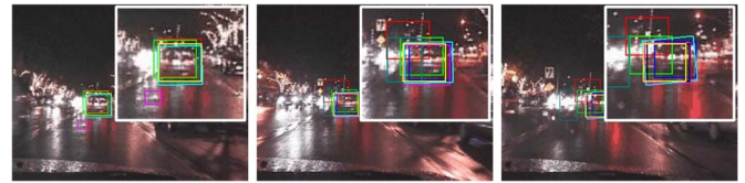
Fig. 7. Comparison on CAR11 . We compare (yellow) “our method with MS” and (black) “our method with FBMS” with (red) the mean shift, (green) the CBWH mean shift, (blue) online boosting, (pink) TLD, (dark green) L1, and (cyan) IVT. Top-right patches illustrate the close-ups.
