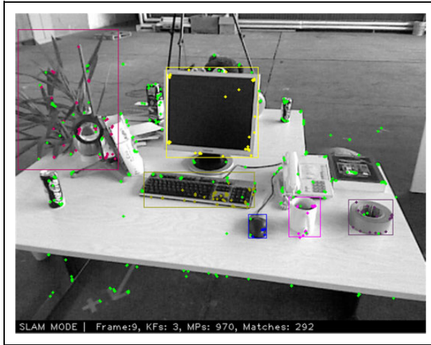
Figure 3. Results of point-object association for an image in fr2/desk of TUM RGB-D data set, where the color of points belonging to the same object is the same as that of the corresponding bounding box.
