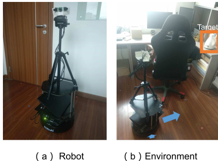
Figure 4: Robot and physical environment. There are three cameras attached to the top of the Robot. The cameras on both sides are at a 45-degree angle to the middle camera.
