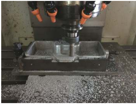
Fig. 18 Finish machining on the sensor cover mounted on the fixture
