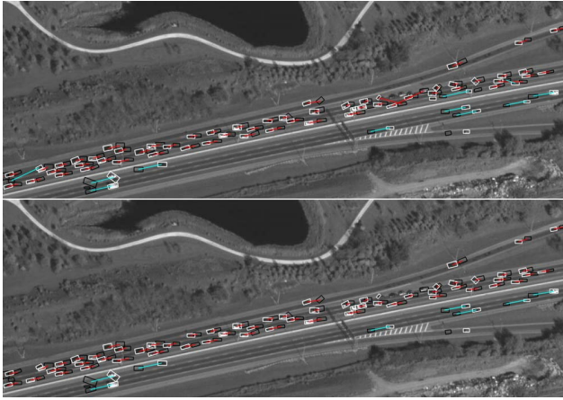
Figure 6. Association results on CLIF (part). Top: tensor method [19] has 6 mismatches; Bottom: our approach has no mismatch; White (black) rectangles: vehicle detections in current (last) frame; Red (green) lines: associations on two orientations.
